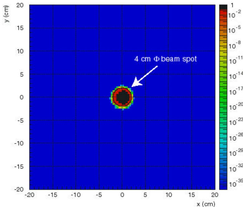
**Figure 3.** Attenuation factors for neutrons of 1 MeV, generated isotropically from the Pb target within a cone of  $1^\circ$ , upstream to 185.5 m (experimental area). The densities of the materials are the real ones and the neutrons were generated with the approximated spatial distribution (from FLUKA simulations).
