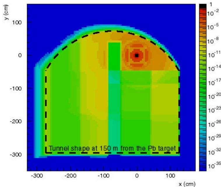
**Figure 1.** Attenuation factors for neutrons of 1 MeV, generated isotropically from the Pb target within a cone of 1°, upstream to 150 m (beginning of the secondary experimental area). The densities of the materials have been divided by 10 and the neutrons were generated with the proper spatial distribution.
