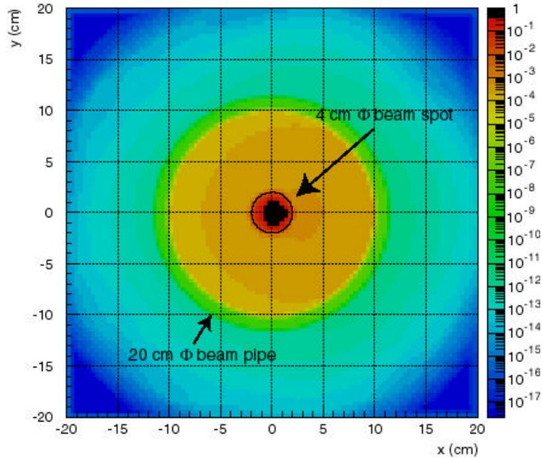
**Figure 2.** Attenuation factors for neutrons of 1 MeV, generated isotropically from the Pb target within a cone of  $1^\circ$ , upstream to 185.5 m (experimental area). The densities of the materials have been divided by 10 and the neutrons were generated with the approximated spatial distribution (from FLUKA simulations).
