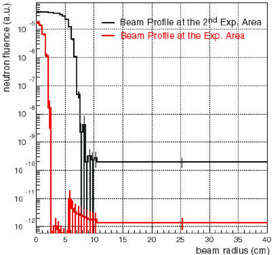
**Figure 6. Radial beam profile distributions at the the 2<sup>nd</sup> experimental area (in black) and main experimental area (in red).**
