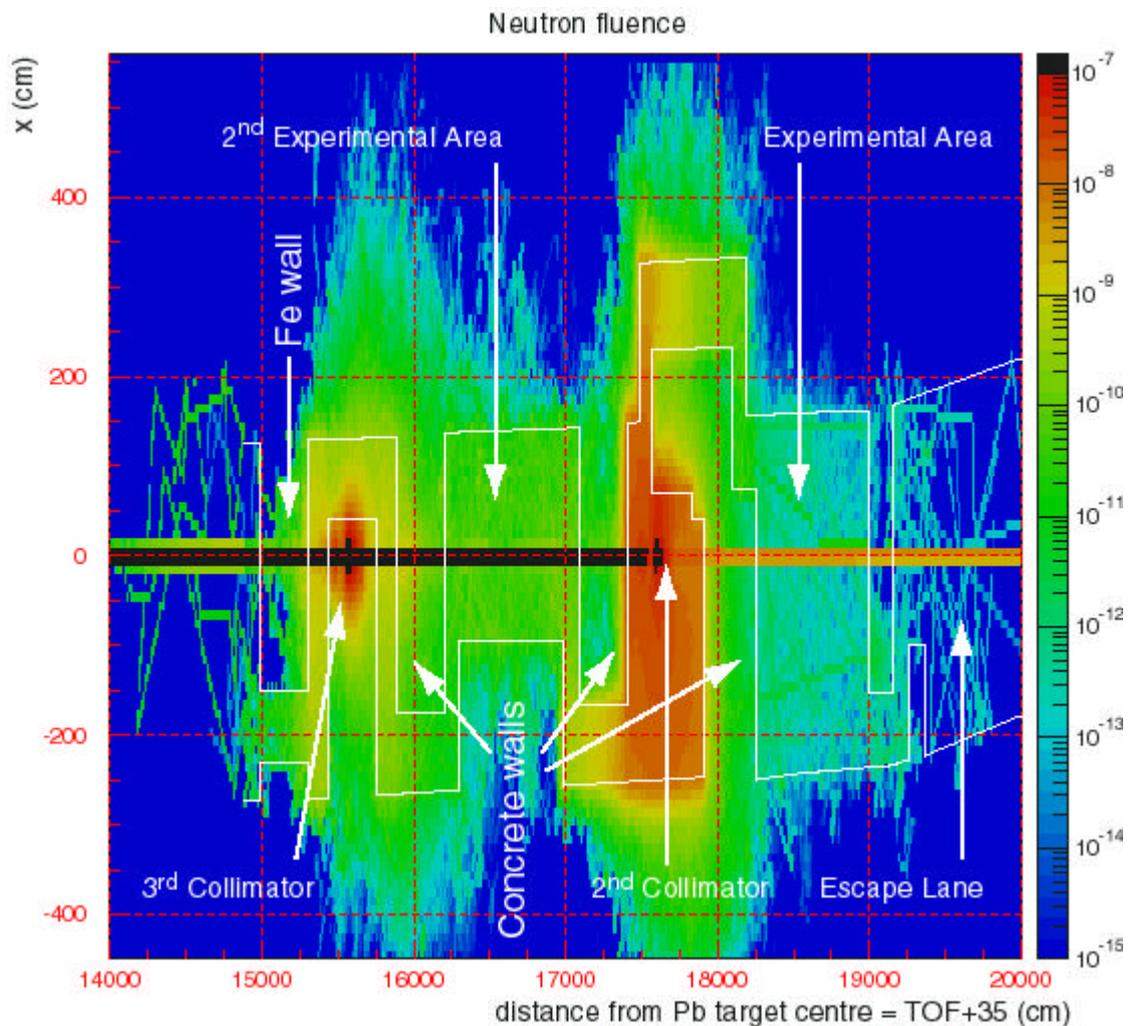
**Figure 2. Neutron fluence distribution along the last 60 metres of the tunnel. The figure represents a bird's-eye view of the nTOF tunnel. Both horizontal (beam axis) and vertical (horizontal tunnel x-axis) axes have been divided in 10 cm substeps. The perpendicular axis (not seen in the plot) corresponds to one single bin between -500 and 500 cm which includes the floor and ceiling of the nTOF tunnel.**
