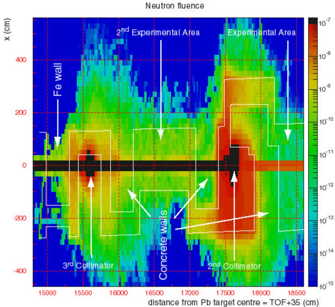
**Figure 3. Neutron fluence distribution between 140 and 186 metres from the centre of the Pb target. The distribution corresponds to a cut on the vertical axis above and below the nTOF tube which neither includes the floor nor the ceiling.**
