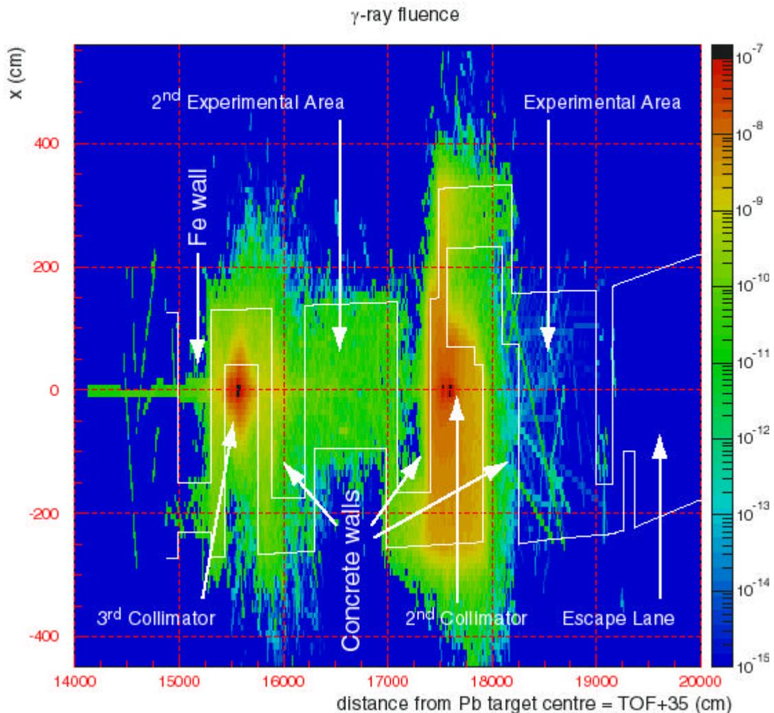
**Figure 4. Neutron-induced gamma ray fluence distribution along the last 60 metres of the tunnel. The figure represents a bird's-eye view of the nTOF tunnel. Both horizontal (beam axis) and vertical (horizontal tunnel x-axis) axes have been divided in 10 cm substeps. The perpendicular axis (not seen in the plot) corresponds to one single bin between  $-500$  and  $500$  cm which includes the floor and ceiling of the nTOF tunnel.**
