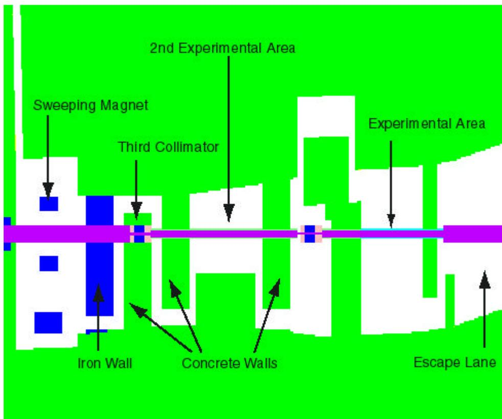
**Figure 1. View of the geometry of the proposed 2<sup>nd</sup> experimental area and main experimental area as defined for MCNPX. Notice that the vertical (x) and horizontal (z) axes are not in the same scale.**
