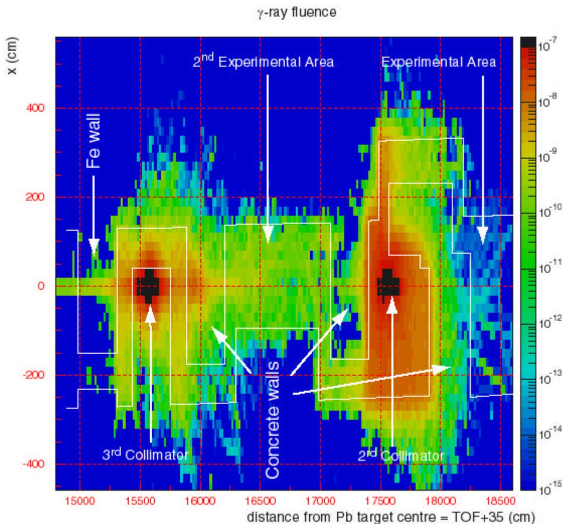
**Figure 5. Neutron-induced gamma ray fluence distribution between 140 and 186 metres from the centre of the Pb target. The distribution corresponds to a cut on the vertical axis above and below the nTOF tube which neither includes the floor nor the ceiling.**
